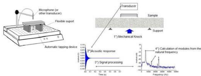
Figure 3 - Scheme of the experimental apparatus used in the resonance frequency test. [7], [8]
