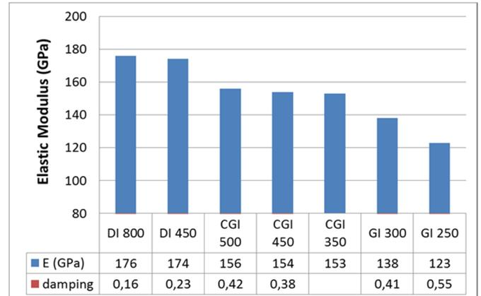
Figure 4 – Elastic modulus and damping capacity of cast irons.
