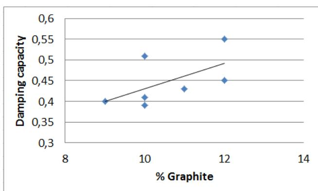
Figure 10 – Relationship between graphite microscopic characteristics and damping capacity in gray irons. Bars with 30 mm diameter. Damping capacity increases with lower eutectic cell number and higher amount of graphite, the opposite trend for elastic modulus and UTS.
