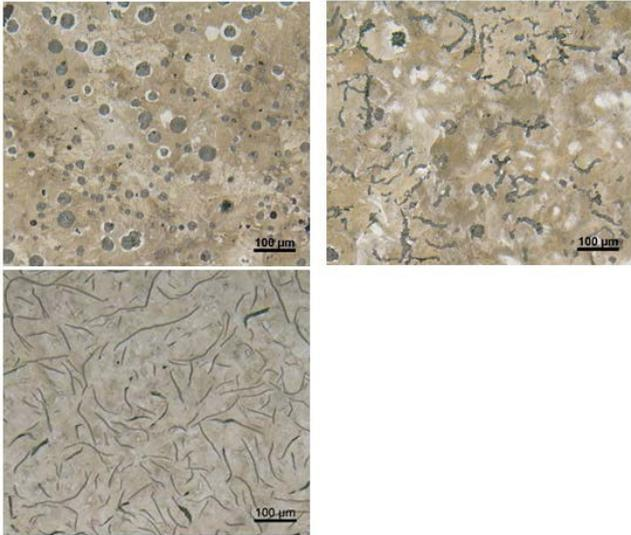
Figure 2– Typical microstructures of ductile iron (grade 800), CGI (grade 450) and gray iron (grade 300), with Nital etching.
