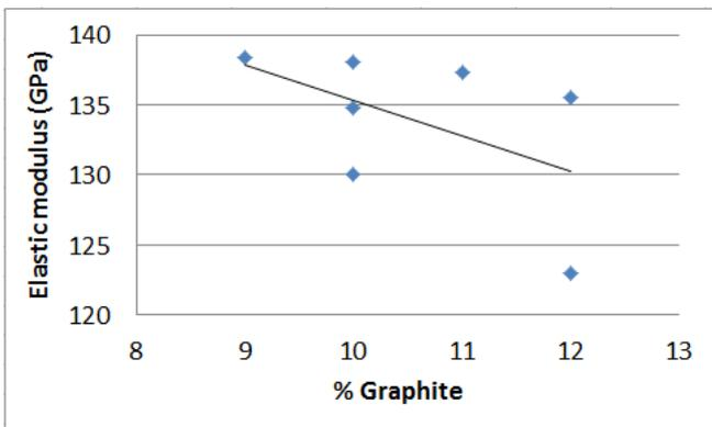
Figure 8 – Relationship between graphite microscopic characteristics and elastic modulus in gray irons. Bars with 30 mm diameter. Elastic modulus increases with higher eutectic cell number, refined graphite and lower amount of graphite, the same trend for UTS.
