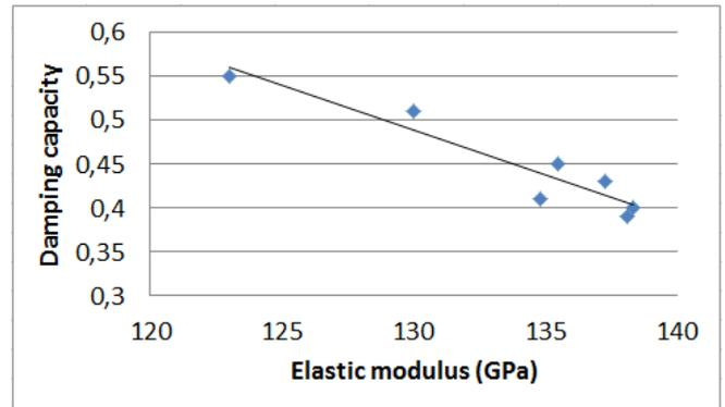
Figure 9 – Relationship between elastic modulus and damping capacity. Inverse relationship.
