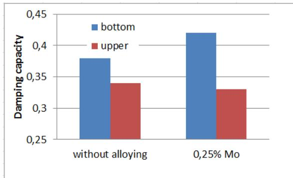
Figure 5 - Results of elastic modulus and damping capacity of CGI samples, in bottom and upper position of the Y block.
